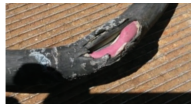
IMAGE C – CUT OUTER SHELL AND SMASHED CONDUCTORS
